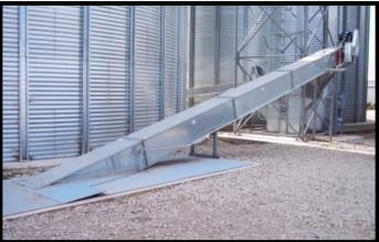
When it comes to continuous conveyors, the drag chain conveyor (also known as the spillage conveyor) is counted among the most tested and important kinds of transport for a wide variety of bulk materials. Our drag chain conveyors are suited for continual horizontal or steeply inclined transport.
